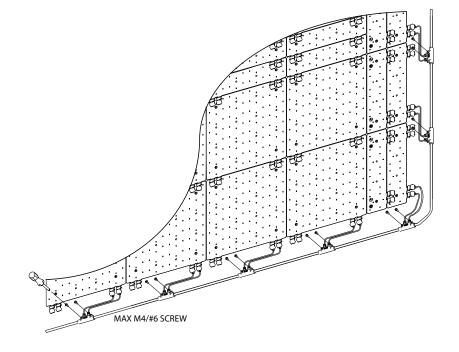
Connect the single wires from each T to one set of connectors on each run. Either set of connectors on the TILE may be used as required.
