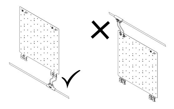
Refer to the project layout drawings to locate the first run of TILE Exterior. Space should be left adjacent to the TILEs for the starter cable.
