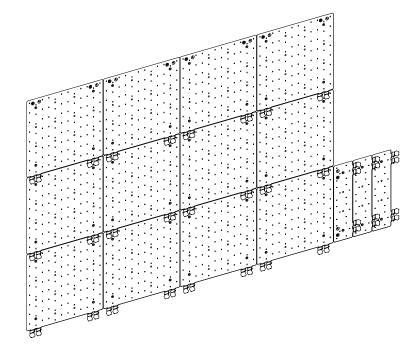
3. Mount and connect the same quantity of the TILE Exterior Fit4 segments alongside each row of the installation.
