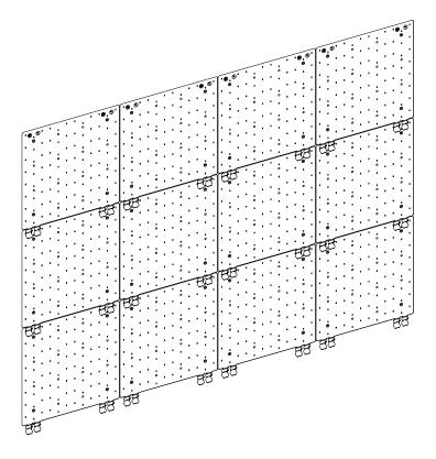
TILE Exterior cannot be cut. For this reason, when installing a run that is <12" (305mm) in width, it is necessary to use Exterior TILE FIT sheets, rotated 90 degrees, to fill the remaining space.
