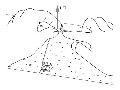
To separate a cable harness from a TILE Exterior piece grip the plastic cover of the tab between the thumb and index and gently pull the moulded head of the wire harness straight out from the connector. Do not lever off the wire as this may damage the connector.
