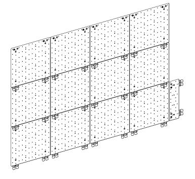
2. If required, connect and mount up to two (2) additional TILE Exterior Fit 4 segments to the first.
