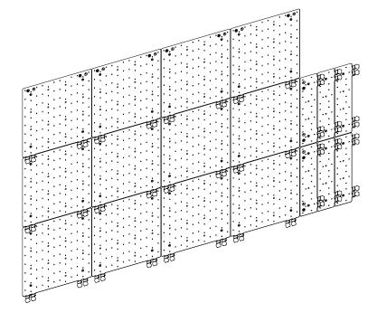
1. Mount the first TILE Exterior Fit4 segment edgeto-edge with the first TILE of the last run with the tabs facing away from the adjacent TILE.
