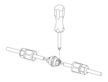
Tighten the housing onto the splice connector body.
