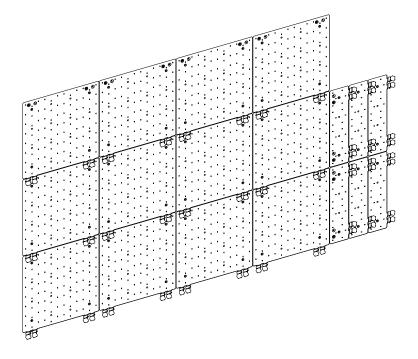
4. If the last TILE of each run was a TILE Exterior Fit segment, use one (1) to three (3) smaller TILE Exterior Fit segments to fill the final space.
